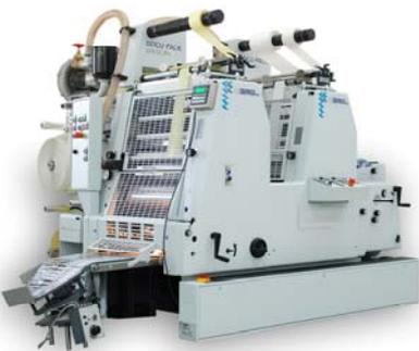
The Docupack from Unigraphica is actually a Heidelberg GTO 52 ZP plus. The offset printing machine with two print units was converted into a sheet-finishing system, which can apply labels or cards to printed sheets from offset or digital printing.
