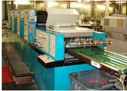
High pile delivery
